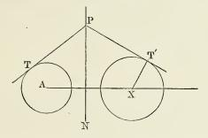
Solution. From the centre A draw an indefinite line AX perpendicular to the line N.
